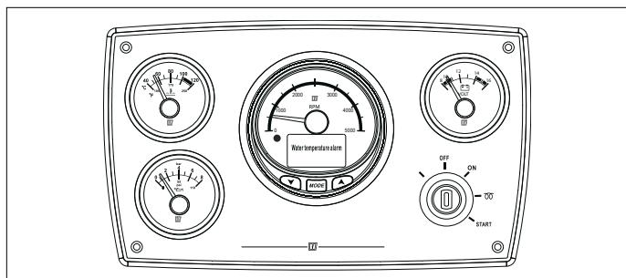
The panel has a built-in audible alarm and can be used as a single, first or second, panel.
