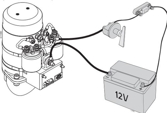
Connect the main power supply cables. ◀
