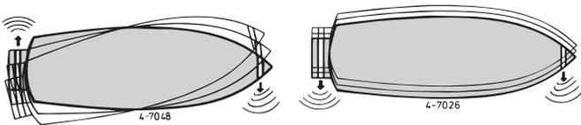
If, in addition to controlling the movement of the bow, the stern of the vessel is required to move sideways, then a second thruster may be installed at the stern. ◀
