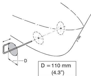
Dependent on the vessel's construction material, cut out the holes by means of a jigsaw or an oxy-acetylene cutter. ◀
