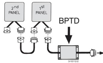
If there are two steering positions, the second control panel can be connected to the first one.
