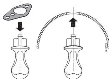
Grease the hole of the intermediate flange and position this flange. Fit the bolts. ◀
