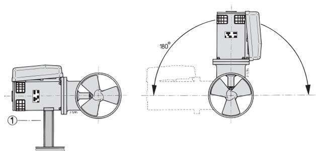
The electric motor can be installed in various positions.
