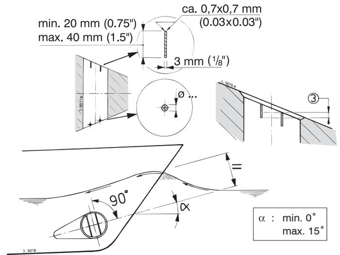
Although the thrust force will be adversely affected, grid bars may be placed into the tunnel openings, for protection of the thruster. ◀
