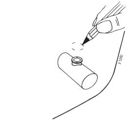
Use the drill pattern supplied, to determine the correct position of the holes to be drilled. ◀
