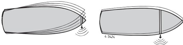
To achieve the optimum performance, position the thrust tunnel as far forward as possible. ◀
