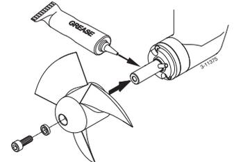
The propeller should run a minimum of 1.5 mm free of the thrust tube wall, all round. ◀
