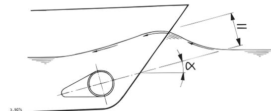
Length 'L' of the fairing should be between 1 x D and 3 x D. This fairing should be embodied in the ship's hull in such a way that the centerline of the fairing will correspond with the anticipated shape of the bow-wave. ◀
