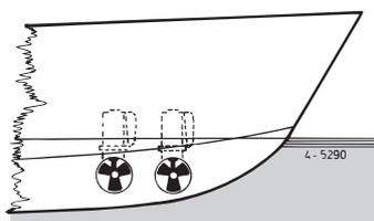
When choosing the location for the thrust tunnel, take the following into account for optimum performance:
