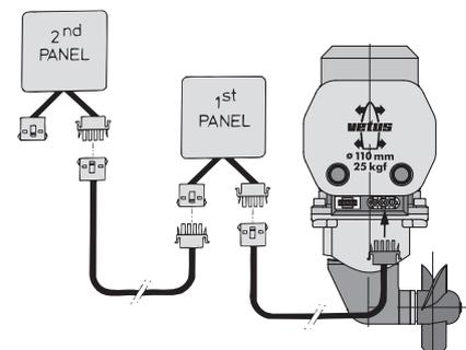
N.B: The colours of the wire cores in the intermediate cable may differ from the wire core colours as used on the bow thruster motor and on the control panel! ◀
