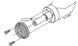
Clean the propeller shaft, grease with 'outboard gear grease' and refit the propeller on the shaft. ◀
