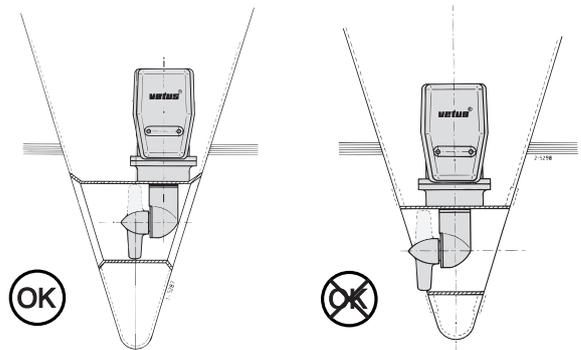
When determining the exact position of the bow thruster in the thrust tunnel, it should be taken into account that the tailpiece may NOT protrude from the tunnel end.
