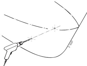
Pass the marking tool (home-made) through both pre-drilled holes and set out the outside diameter of the thrust-tunnel to the hull. ◀
