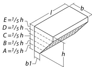
As an example a tank with a partially sloping side
