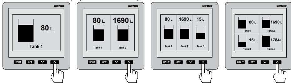
Scroll down through tanks in the screen when there are more tanks than can be shown simultaneously in the screen:
