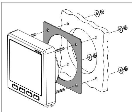
Cut holes in the instrument panel or a bulkhead using the template supplied. Fit the display instrument using the 4 threaded studs and nuts supplied. Make sure that the packing is positioned correctly between the instrument and the panel or bulkhead.
