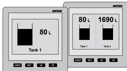
The settings for the tanks can be made on either of the display instruments and then also apply automatically for the other instrument.
