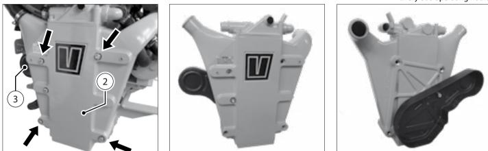
• Remove the 4 bolts and remove the charge air cooler (2) together with the drive belt cover (3).
