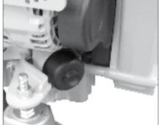
14 Removing the oil filter
