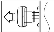
Press the green key (■) on the remote control briefly. The battery main switch will now be switched on. The light on the remote control will come on.
