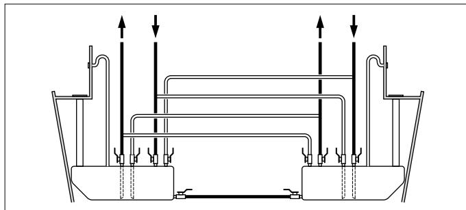
Distribute the tanks, that is the weight, uniformly over the ship.
