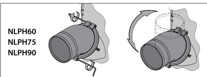
Loosen the bolts before turning the hose connections! Tighten the hose connections to a torque of 1 Nm (0.74 ft-lb, 142 oz-in).
