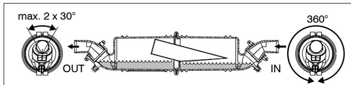
For a proper working it is essential that the OUT part of the housing and both the inner parts are placed in the positions as shown in the illustration. A deviation of maximum 30° to either side is permitted. The IN part of the housing may be placed in any position.
