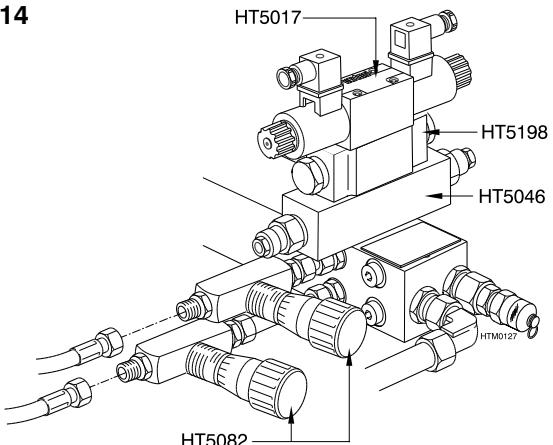
When putting into operation, the flow should be set using the flow control valve (HT5082). The flow is related to the speed of the mast-lowering system.
