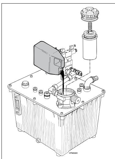
A combined thermometer/depth gauge is fitted to the tank.
