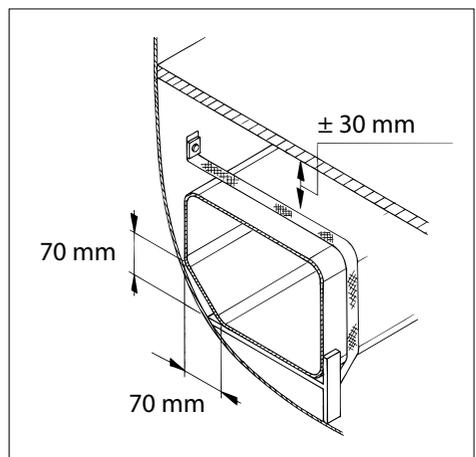
Make sure the tank has a sufficiently secure foundation on which to install it and secure it properly.
