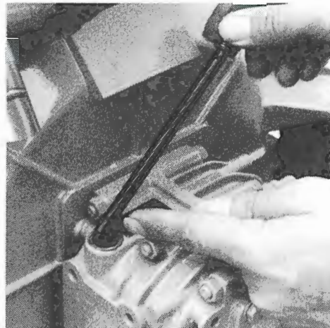
Olie peilen. Checking the oil level.
