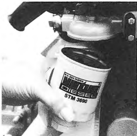
Brandstoffilter demonteren. Fuel filter removal.
