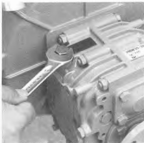
Losnemen peilstok. Unscrewing the dipstick.
