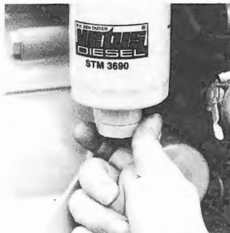
Waterafscheider aftappen. Draining water separator.
