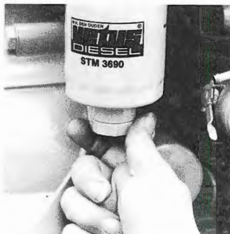
Waterafscheider aftappen. Draining water separator.
