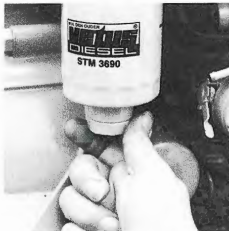
Waterafscheider aftappen. Draining water separator.
