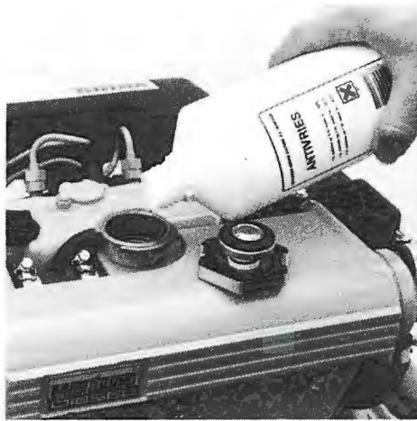
Vullen koelsysteem. Filling of cooling system.
