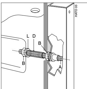
Screw 2 bolts (B) onto the threaded studs and screw the footplate (N) over the threaded studs. Fix the footplate (N) with one nut (B). Screw the adjustable feet into the frame.
