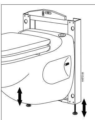
Tighten the nuts (B) to fix the adjustable feet to the frame. Remove the pot from the frame.
