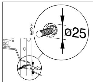
Fit a hatch opening in the false wall so that the ball valve in the supply pipe will always be accessible without having to dismantle the toilet pot.
