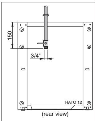
If there is already a pressurised water system on board the supply hose can be connected to this system. The pressure must be at least 1.5 bar; this is the minimum pressure required to allow the toilet to function properly.
