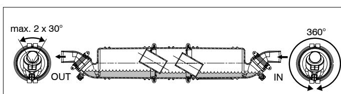
For a proper working it is essential that the OUT part of the housing and both the inner parts are placed in the positions as shown in the illustration. A deviation of maximum 30° to either side is permitted. The IN part of the housing may be placed in any position.
