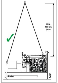
The lifting hooks are engineered only to lift the generator set without any extra weights!
