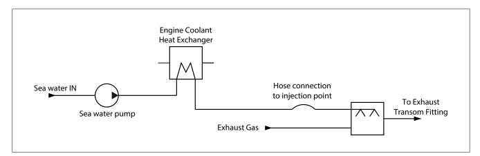
The engine heat exchange circuit is represented in the block diagram below:
