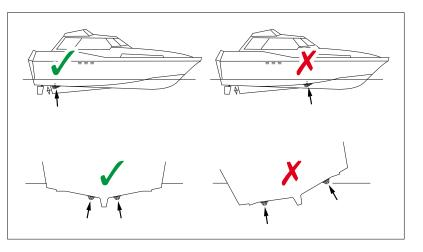
2 Place the water scoop with the opening facing forwards or backwards depending on the type of boat:
