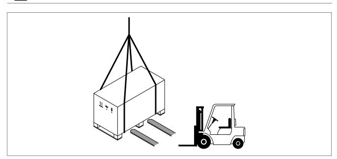
When you install the generator set on the boat after opening the packaging always follow the hoist instructions below.
