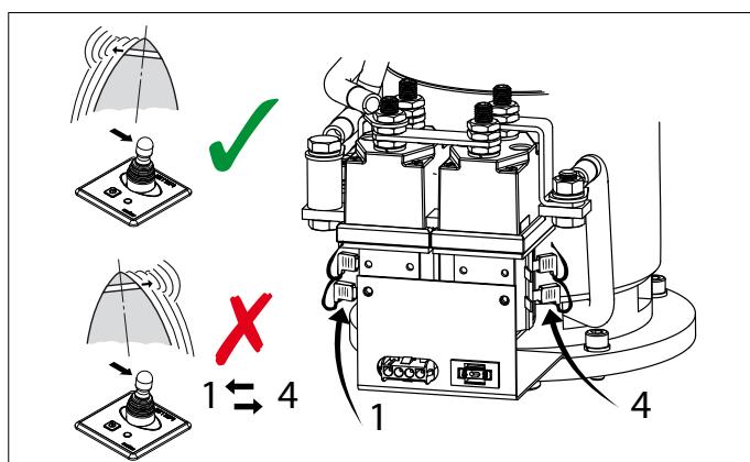
If test running shows that the thrust direction of the bow thruster is not the same as that shown by the direction switch on the control panel the blue (no.1) and the white (no.4) wires on the relay must be changed round.
