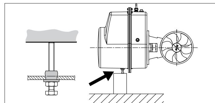
If the motor is positioned horizontally support is absolutely essential.
